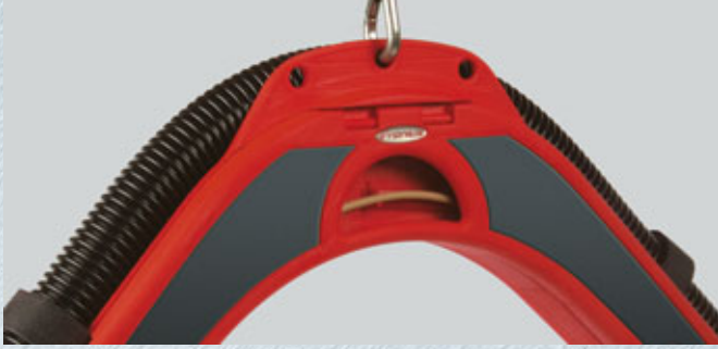
The wire buffer decouples the front and rear wire-drives from one another and ensures smooth wire travel.
