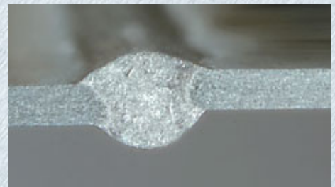
Butt-weld, without weld-pool backing support, on 0.8 mm AlMg3 sheet.
